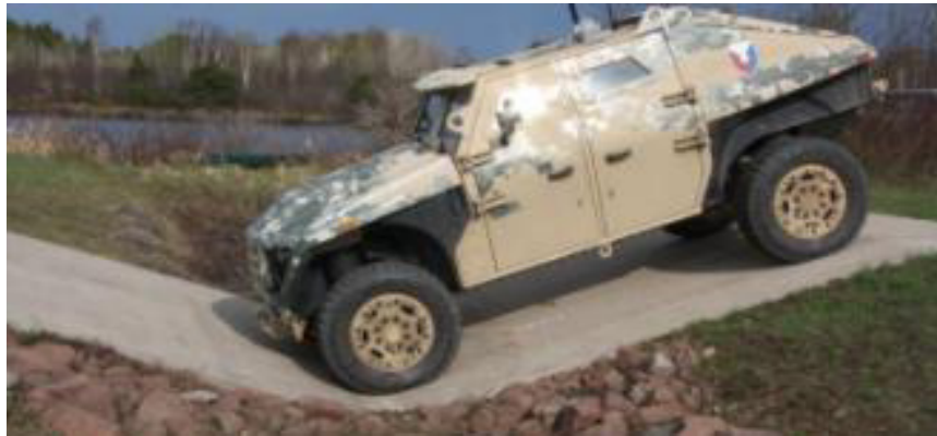
Figure 2-8: V-Ditch Performance, Go/No-Go.
